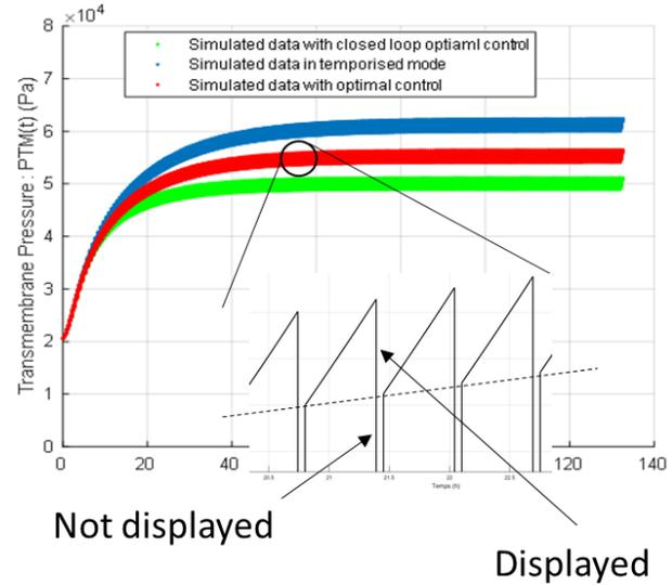
Figure 6. TMP simulations using the three control strategies with constant input concentrations (constant phase length open-loop control in blue, open-loop optimal control strategy in red and adaptive – closed-loop – control strategy in green)
