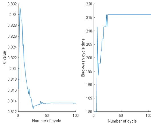
Figure 4. Adaptation of the optimal lengths of the filtration and backwash phases in the presence of unknown constant input substrate concentrations. On the left the ratio ( $t_f/t_{bw}$ ), on the right  $t_{bw}$  (in seconds)
