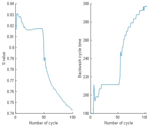
Figure 5. Adaptation of the optimal lengths of the filtration and backwash phases in the presence of an unknown magnitude step in the input substrate concentrations. The ratio ( $t_f/t_{bw}$ ) is plotted on the left and  $t_{bw}$  on the right (in seconds)
