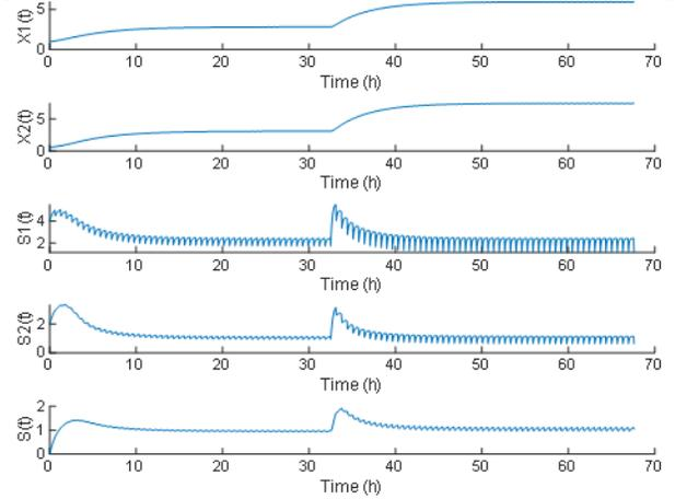
Figure 3. Open-loop simulations of the MBR with step input concentrations.  $S$  stands for  $S_p$ . ‘‘Oscillations’’ (high variance) observed on some signals are due to the succession of filtration/backwash cycles which have more important repercussions on some variables than on others.
