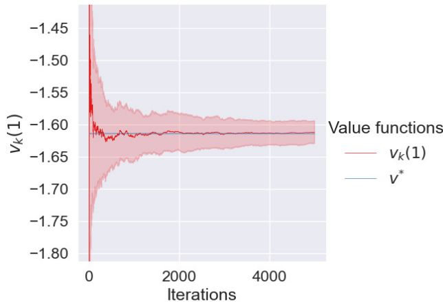
(b) The estimation of the cost-to-go function for observable state 1 in each algorithm iteration.
