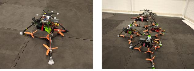
Fig. 1. A single module (left); the four-module assembly (right).
