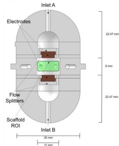
Fig.1 Bioreactor design: vertical cut view, illustrating parallel electrodes set up, upper and bottom inlets and inlet flow splitters [3].
