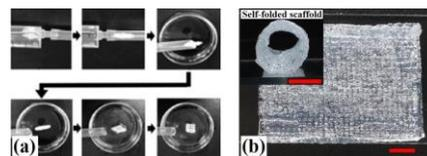
Fig.3 4D printing of TE scaffolds: (a) shape recovery of a 4D printed scaffold [14], (b) self-folded tubular scaffold [15].
