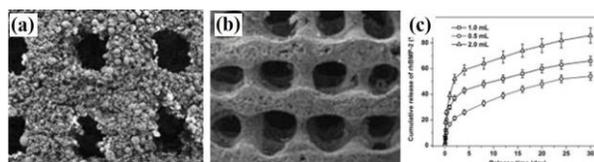
Fig.2 3D printed scaffolds: (a) scaffold formed by SLS [7], (b) scaffold formed by extrusion [11], (c) growth factor release from scaffolds [11].
