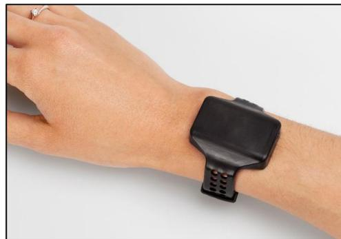
Figure 1. *PulseWatch* device attached to the wrist. The device includes three PPG channels (green, red and infrared) as well as an accelerometer sensor.
