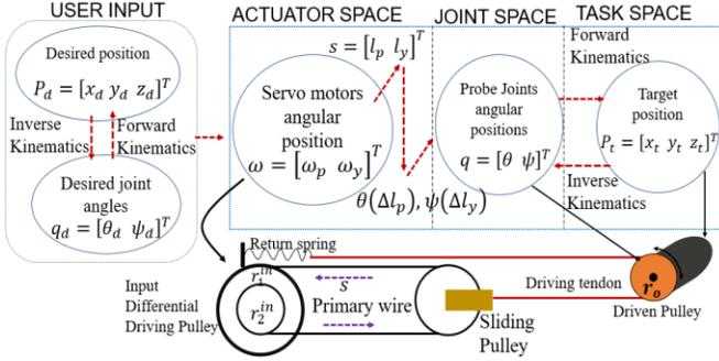
Figure 3. Kinematic mapping
