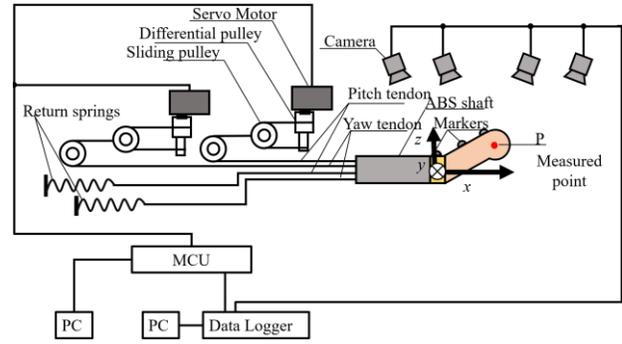
Figure 5. Experimental setup for measuring position  $P$ .
