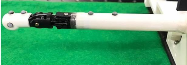
(b) Palpation probe prototype
