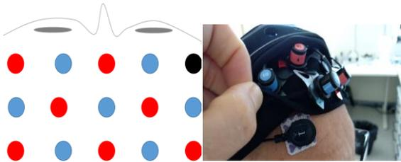
Figure 1. Optical sources (red points)/detectors (blue points) and EEG electrode positions (black point).
