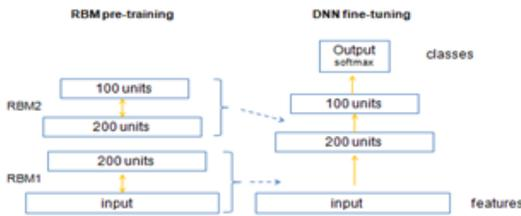
Figure 4: Deep classifier: Restricted Boltzman Machine (RBM) and Deep Neural Network (DNN).
