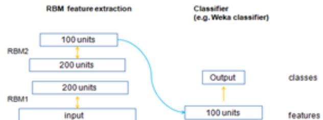
Figure 1. Structure of deep feature extractors: Restricted Boltzman Machine (RBM) with classifier.
