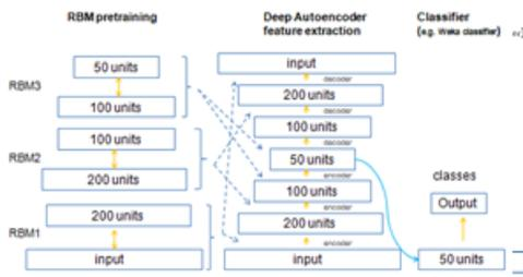
Figure 3: Structure of deep feature extractors: Deep Autoencoder with classifier.
