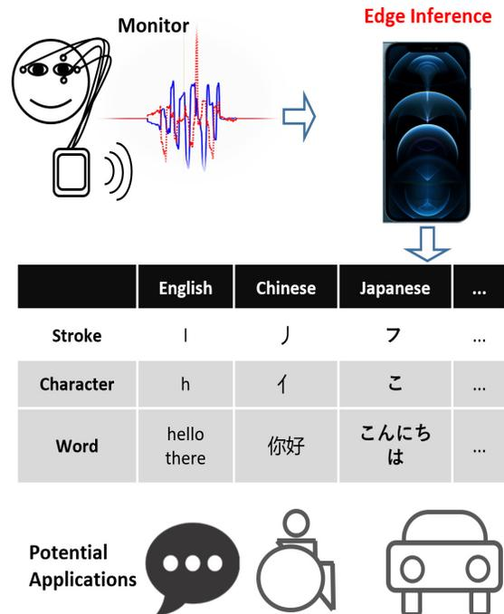
Fig. 1 A systematic concept of how human big data decoding on the edge can enable promising applications. Here we take special interest in decoding the brain visual dynamics, i.e., the Electrooculogram (EOG) signal, for the voice-free communication application for ALS patient.
