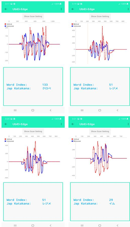
Fig. 4 Further screenshots of UbiEi-Edge about visualization and decoding of the visual dynamics, which demonstrates the effective illustration of the real-time visual dynamics and the deep learning-based inference results.
