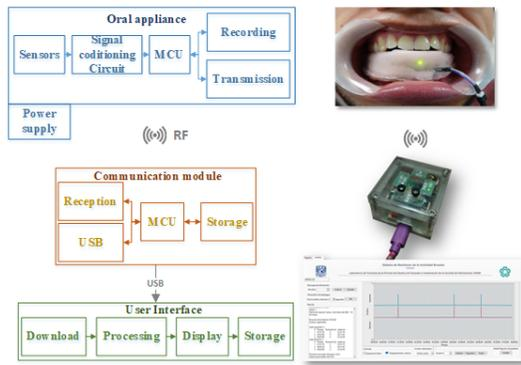
Fig. 1. Block diagram of the Bruxist Activity Monitor System (BAMS).
