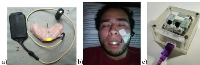
Fig. 2. a) Oral Appliance: Occlusal splint (1), Battery (2), and Magnet (3); b) Test subject wearing the Oral Appliance during a recording session; c) Communication Module.
