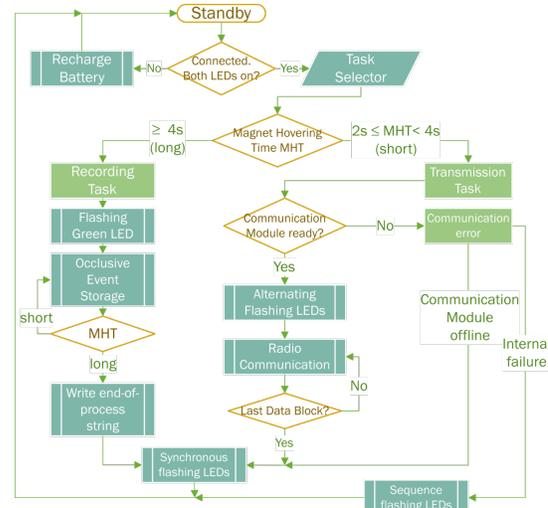
Fig. 4. Oral Appliance diagram flow.
