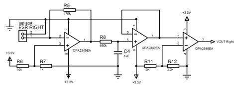
Fig. 3. Signal Conditioning Circuit (right channel).
