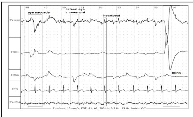
Figure 3. Pipeline cleaning for eye movements and heartbeat artifacts. From top to bottom: FPz raw data, EOGv, EOGh, ECG, FPz cleaned using ICA-MARA+. Subject S1, scenario 3, Fpz.
