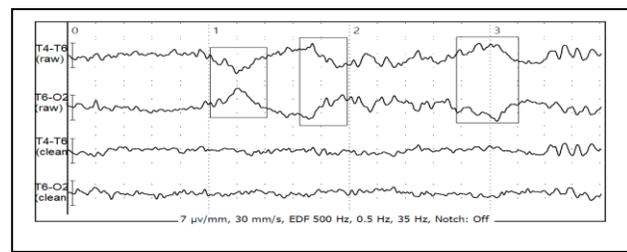
Figure 5. Channel artifacts cleaning. From top to bottom: raw data (T4-T6), raw data (T6-O2), ICA-MARA+ (T4-T6), ICA-MARA+ (T6-O2). Subject S1, scenario 3, derivations T4-T6, T6-O2.
