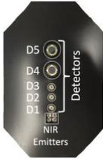
Figure 1. Optical Probe.
