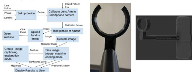
Figure 1. (Left) The function block diagram describes the function between input and output. (Right-top) Complete CAD design for the iPhone 11. (Right-bottom) Real camera view of lens holder.
