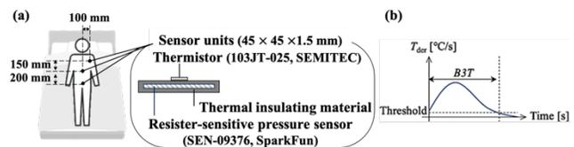
Figure 1. Outline of a measurement system installed in the bed sheet (a) and the definition of body temperature transit time ( $B3T$ ) (b).
