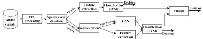
Figure 1. A block diagram of the proposed analysis system
