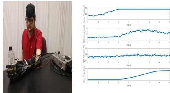
Figure 1. (Left) Complete EEG and EMG-controlled hand exoskeleton system. (Right) Averaged signals for one healthy user during exoskeleton-assisted hand extension. From top to bottom: BCI2000 cursor position for a 1D CursorTask, EDC activation, FDS activation, and motor position.
